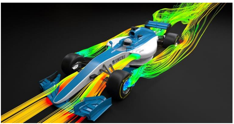
Computational analysis of aerodynamics on F1 car. Source: https://www.simscale.com/blog/front-wing-f1-car-optimize/
