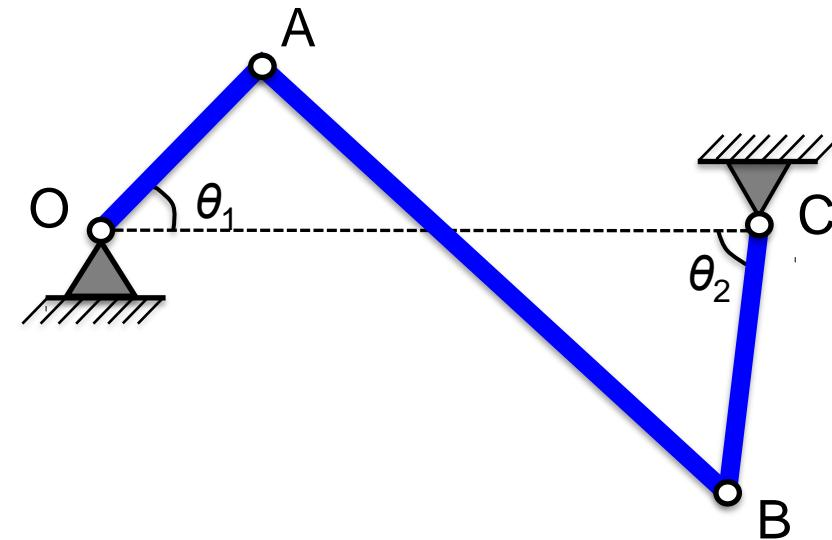
Constrained Systems: some E.o.M. used for calculating reaction forces.
