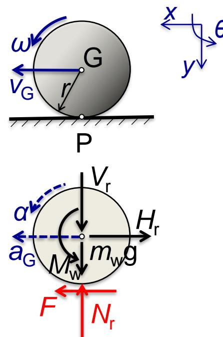
$$x_G(t) = \theta(t)r, \quad \dot{x}_G(t) = \dot{\theta}(t)r, \quad \ddot{x}_G(t) = \ddot{\theta}(t)r$$
