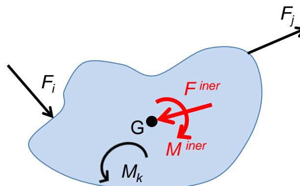
$$\rightarrow^+: \Sigma F_x - F_x^{inertia} = \Sigma F_x - m_G a_{G,x} = 0$$
