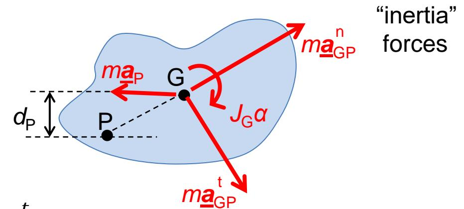
$$\underline{a}_G = \underline{a}_P + \underline{a}_{GP}^n + \underline{a}_{GP}^t$$
